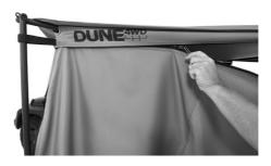
3. **Wall Configuration**: Extend Dune Tapered Wall with Window and Stove Jack, peg-out to secure, refer to below.
