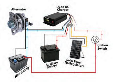
\*Example installation diagram showing wiring colours used for Dune 4WD DC to DC chargers
