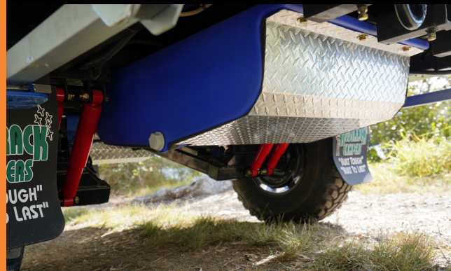
120L Foodgrade poly underfloor water tank with aluminium tank guard & 12v pump plumbed to kitchen. 50L Foodgrade poly water tank with aluminium tank guard plumbed to drawbar to service ensuite.
