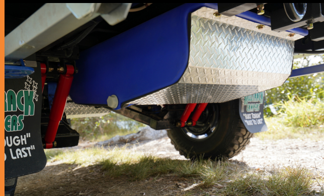
Water storage: 160L Foodgrade poly underfloor water tank and 50L Foodgrade poly underfloor water tank with aluminium tank guard and 12 volt pump plumbed to kitchen.
