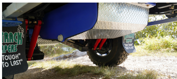
Water storage: 120L Foodgrade poly underfloor water tank with aluminium tank guard & 12v pump plumbed to kitchen. 50L Foodgrade poly underfloor water tank with aluminium tank guard & 12v pump plumbed to drawbar to service ensuite. Manual changeover valve to swap water tanks.
